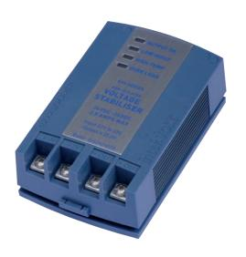
SVS is a power conditioning device without the galvanic isolation. If you don't require DC-DC isolation then the SVS is the cost effective solution for your application. The SVS is a common negative device for 12 and 24VDC transport applications. It will protect your in-vehicle/vessel electronic equipment from a range of voltage issues including dips, spikes, and sustained low and high voltage transients.
