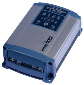
The isolated version ensures complete DC - DC electrical isolation, that is, no common connection between the input and output whatsoever. Isolated converters will eliminate line interference, increase electrical safety with improved circuit protection and reduce voltage transients. This means peace-of-mind when connecting sensitive and often expensive, high-end electronic equipment to the output.
